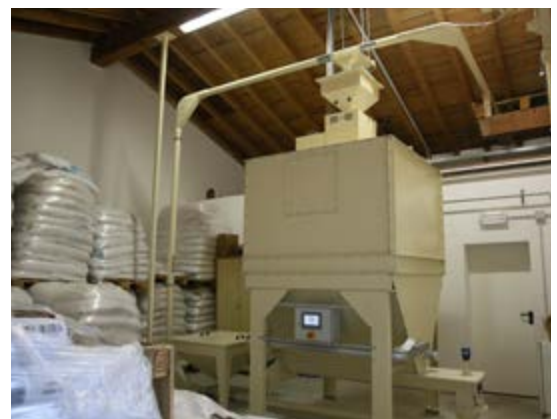
Automated milling and mashing plant, capacity 1 ton
